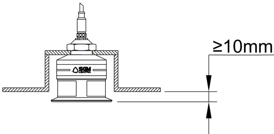
PTU50-51-56 can be installed in an extension pipe to turn away the sensor from the maximum level point. The extension pipe must be flat and without joints (welds, etc.), also, the pipe terminal part must be cut at 45° and with the borders without burr.
